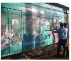
DURING: Due to the size of the project the GRS solution was spray applied for easy application.
