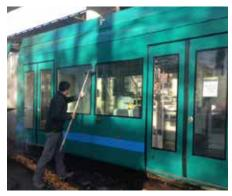
AFTER: Rather than take the rail car out of service for several days to strip and repaint this rail car, was cleaned with the GRS non-toxic solution and back in service within two hours.
